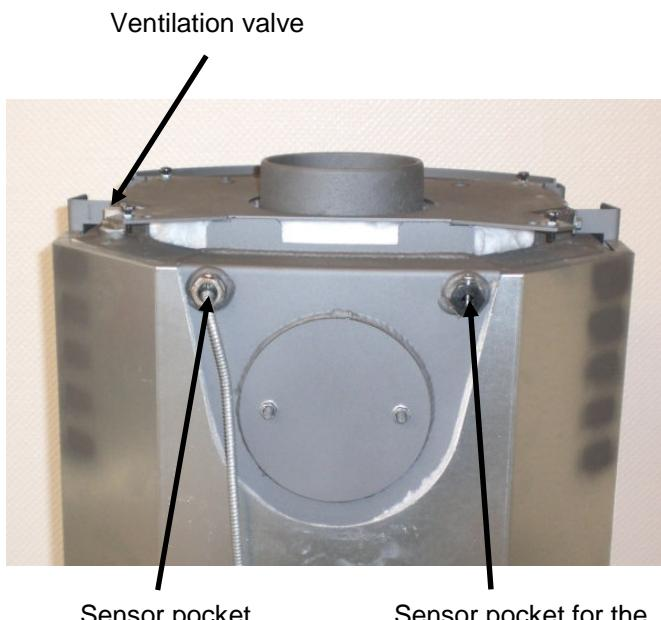
The rear panel of the oven must be removed in order to install the temperature sensor for the water heat exchanger. Slide the temperature sensor into the right-hand thermometer pocket and secure it using the threaded screw.
